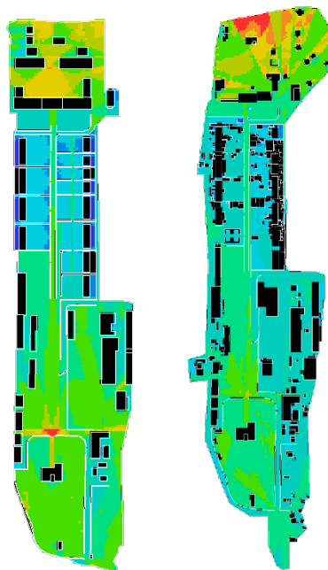
Figure 6. VGA analysis – Integration of Roça Agostinho Neto: original layout (left) and present-day layout (right)
