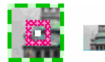
Figure 3. Scale invariant algorithm. Green dashes square: expanded area by s=2.2 (55x55). Pink crosses square: original feature patch ( n=25 , 25x25). White square (center): processed area (7x7). The right image represents the rescaled final patch.
