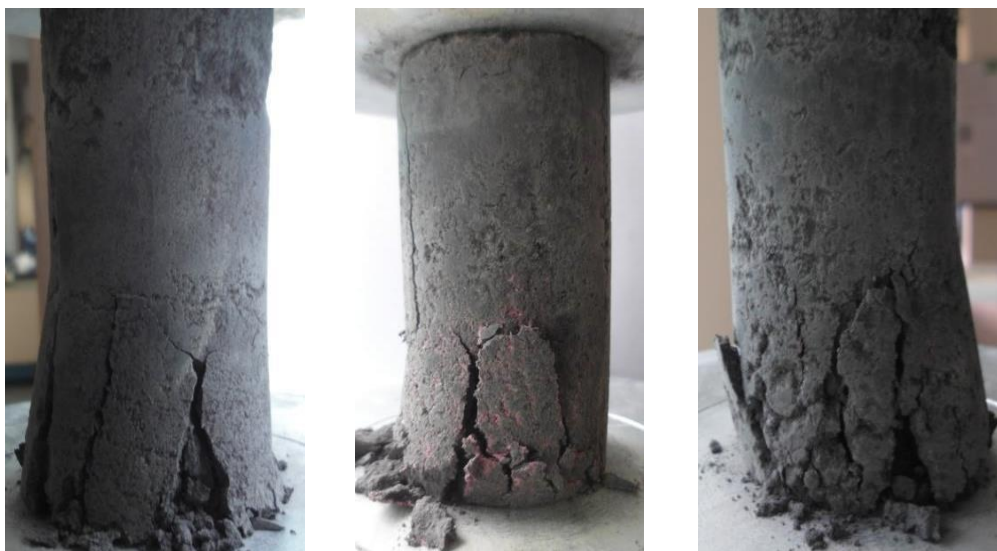
Figure 6: Examples of cracks formation in the mixture of clay-cement-rubberchip
