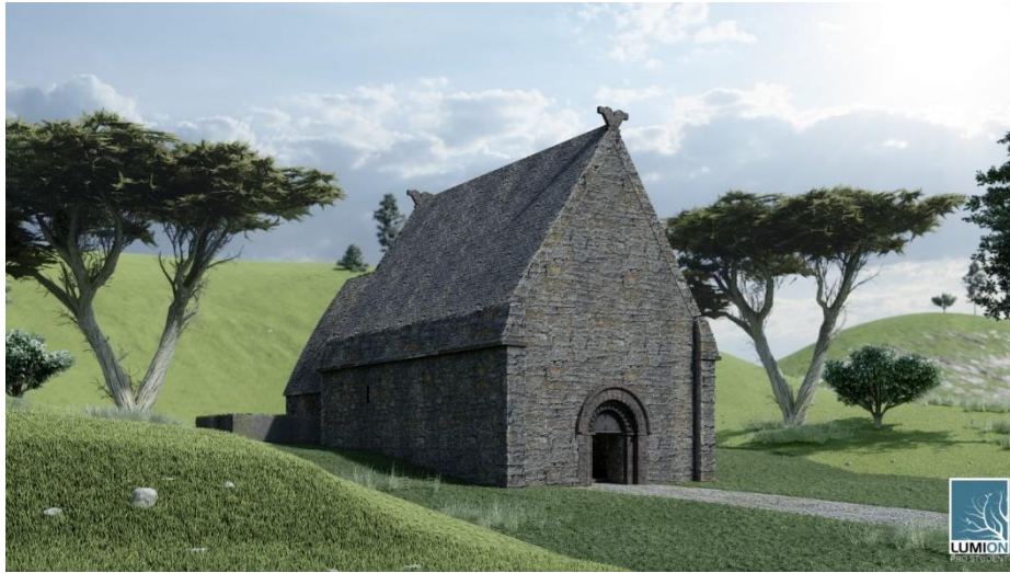
Figure 15: The HBIM model of Kilmalkeader textured and the landscape model added in the software platform Lumion as VR experience of the site
