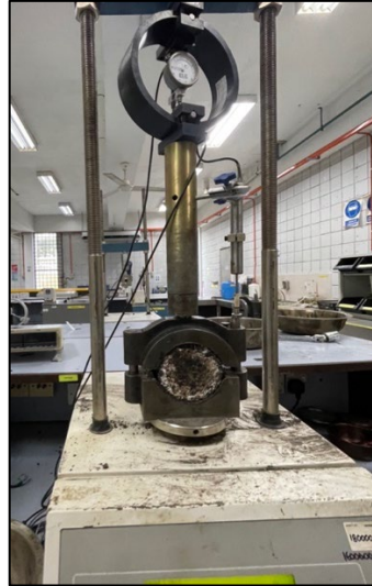
FIGURE 3.11 Marshall stability testing device
