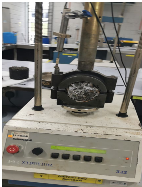
Figure 3.3: Marshall Stability Flow Test Machine
