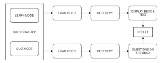
Figure 56. System Architecture
