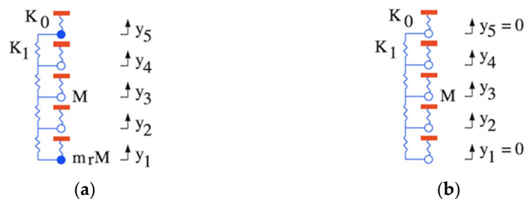
Figure 3. Lumped models of Figure 1b, with (a) mass loaded and (b) fixed end elements.
