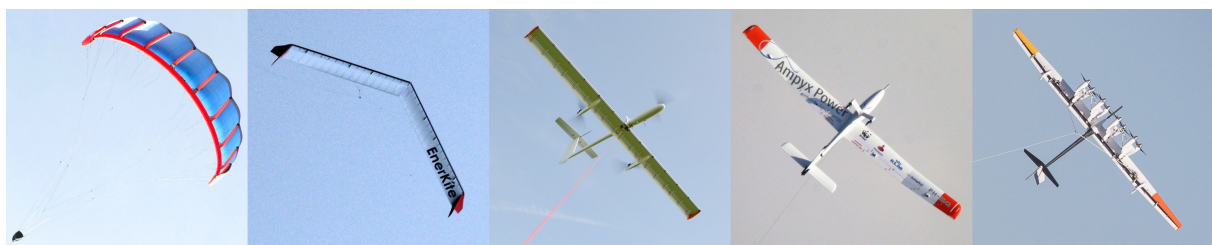
Figure 1. Selected AWE systems currently in development: Kitepower, EnerKite, TwingTec, Ampyx Power and Makani Power (from left to right), generating up to 600 kW per single system.
