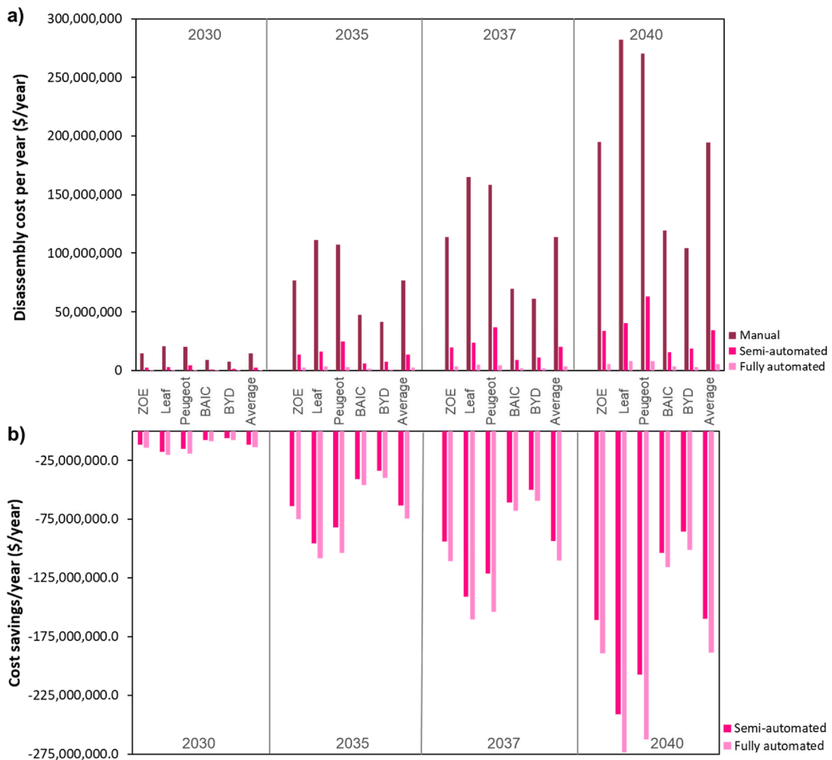
Fig. 5. a) Disassembly costs (in US$) caused by dismantling the predicted amount of EoL battery packs in year 2030, 2035, 2037 and 2040. b) Cost savings (in US$) generated by shifting from manual to semi- and fully automated disassembly.
