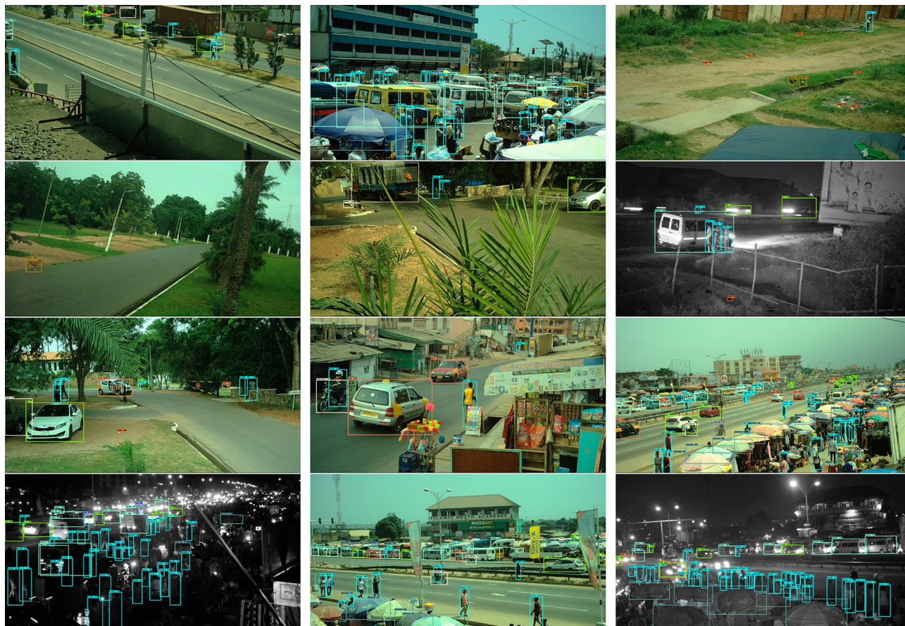
Figure 2. Objects identified in example images. Each identified object is bounded by a box, coloured by object type. The number next to the object's name shows the final layer's activation score for the given object's classifier, which may be heuristically interpreted as the network's confidence score in its prediction. "Truck" refers to pick-up truck, "Bowl" refers to cooking bowl/pot, "Stall" refers to market stalls and "Stove" to cookstoves of the type found in markets.
