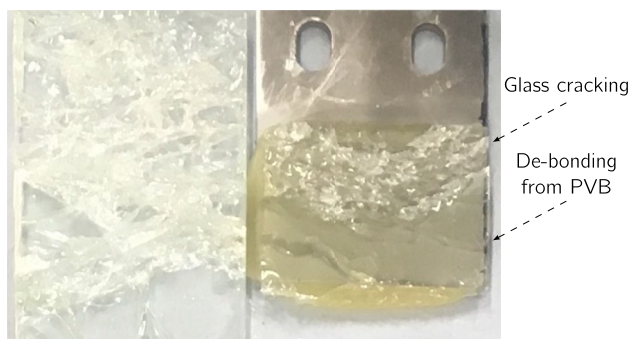
Fig. 14 Delamination failure of specimen with 2.28 mm interlayer tested at 10 m/s (specimen no.18) – side 1
