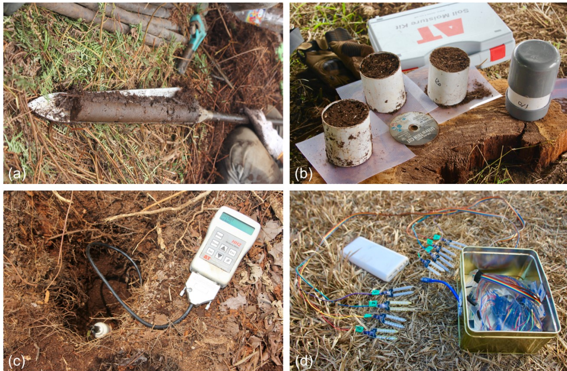
Figure 2.4 Instruments used in peat soil sampling and moisture content monitoring in the experiment. (a) Russian corer, (b) PVC tubes, (c) Delta-T SM150T soil moisture sensor, (d) Arduino soil moisture monitoring system.
