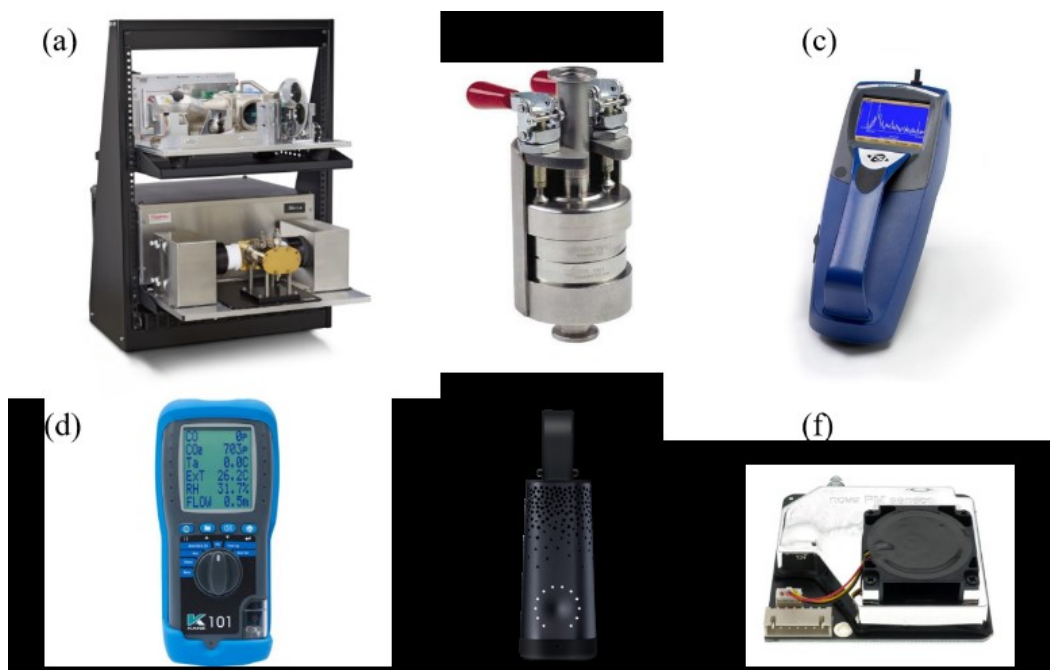
Figure 8.2 Photos of the devices used in this study. (a) Thermo Scientific Nicolet iG50 Fourier-transform infrared spectroscopy (FTIR). (b) Dekati 4-stage PM cascade impactor. (c) TSI DustTrak DRX handheld aerosol monitor. (d) KANE101 indoor air quality analyser. (e) Plume Labs FLOW 2 air pollution sensor. (f) Nova SDS011 PM sensor. The unit sizes of all devices are listed in Table 8.1.
