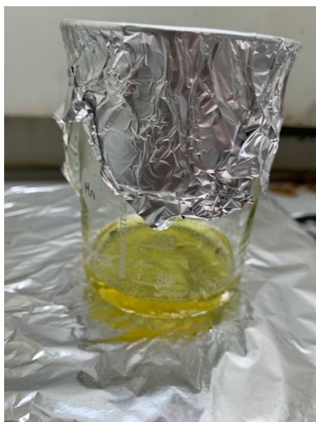
Figure 9-2. Images of the \text{Ca}_2\text{MnO}_4 synthesis process showing a) formed gel of metal nitrate solutions and b) final powder state.
