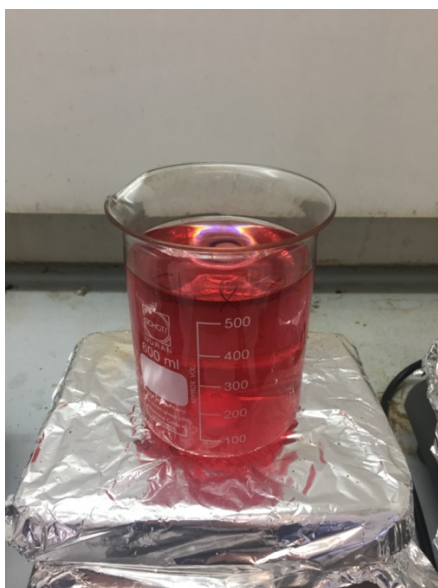
Figure 6-2. a) Stirring solution of Sr, Co and Sb nitrate salts in citric acid, b) Subsequent gel formed upon polymerisation.
