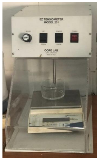
Figure 3-25. EZ Tensiometer (Model 201, USA).
