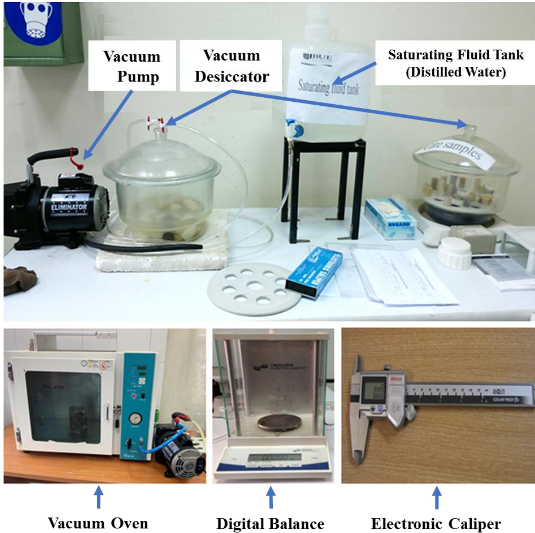
Figure 3-39. The apparatus used in the core saturation process.
