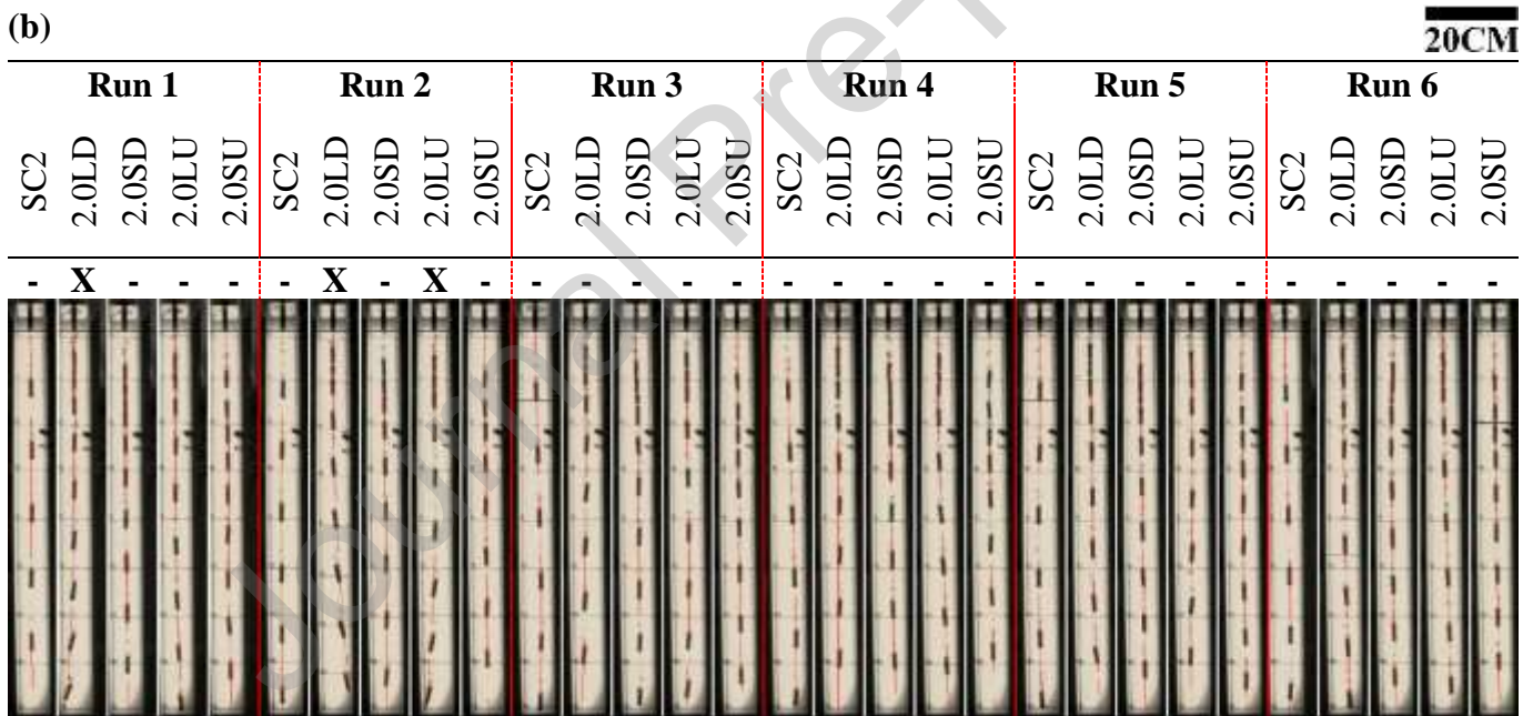
Figure 7: Trajectories of free-falling cylinders at 450^{\circ}\text{C} . As the vapour layer thickens around the cylinders – topological difference in surface finish become increasingly irrelevant. Only cylinders 2.2LD, 2.0LD, and 2.0LU retain free-fall instabilities. X symbol denotes the cylinder hitting the wall.
