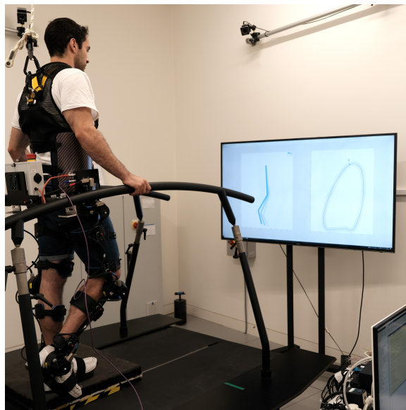
Fig. 1: Data collection setup: A healthy subject performing a trajectory tracking task while wearing a lower-limb exoskeleton.
