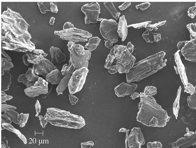
FIG. 1. Scanning electron microscopy image of the Timcal Timrex KS5-75TT graphite particles used in this study obtained using a Zeiss EVO LS15 with an accelerating voltage of 10kV.
