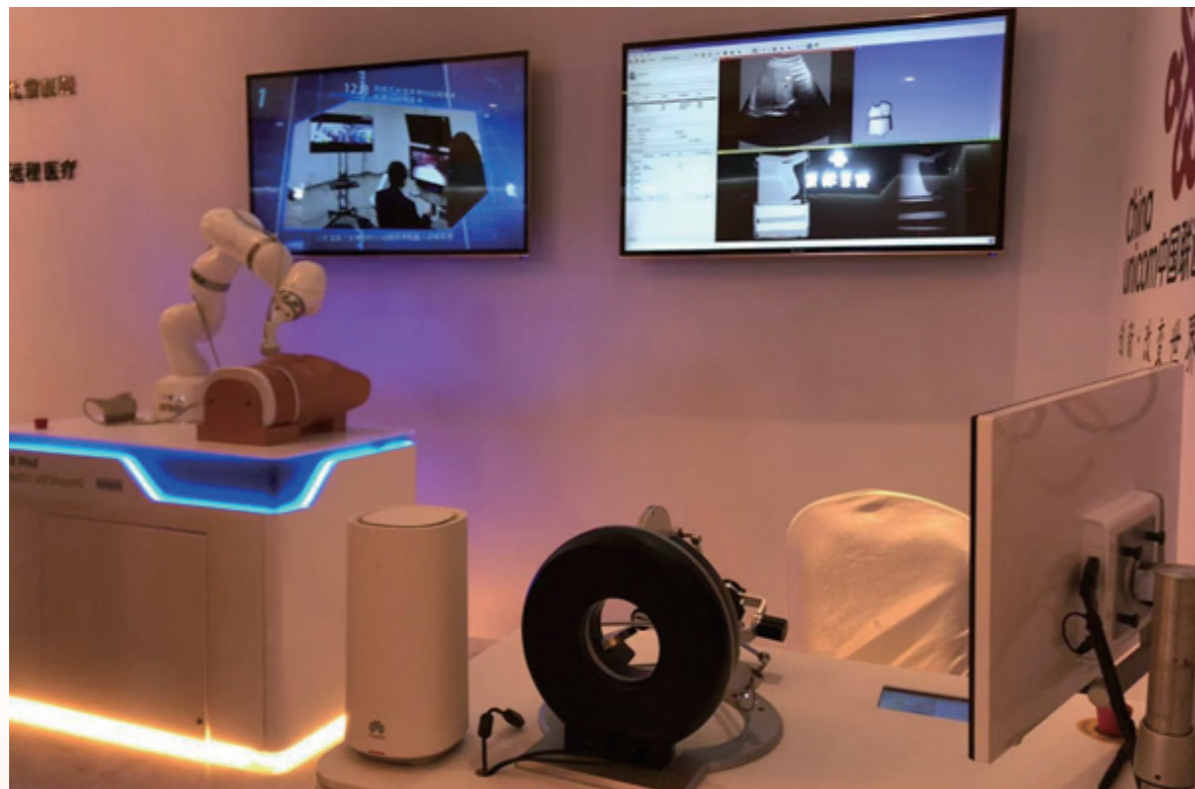
Figure 8: An ultrasound tele-manipulation demonstrator. The patient side of the system consists of an ultrasound transducer attached to a LBR Med robot arm (background), the clinician's workstation consists of a monitor and a haptic input device that renders the forces measured by the robot (foreground). Both systems are connected using a 5G connector (left of the input device)
