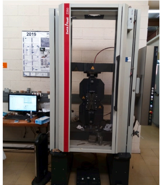
Fig. 2. Zwick/Roell Z250 tensile testing machine.
