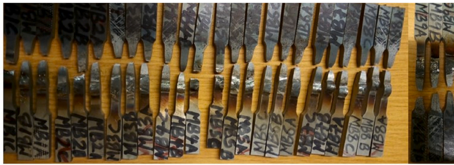
Fig. 4. The fractured tensile specimens.
