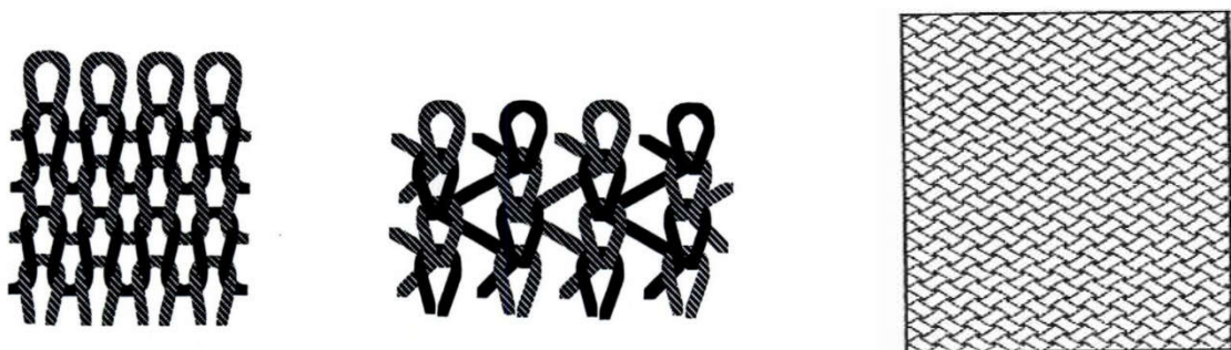
Figure 3.5 (from left) Schematic of weft knit, warp knit, braided fabric
