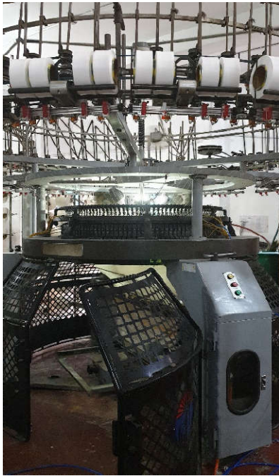
Figure 10.2 Circular knitting machine Source: Author (2020) in field visit of case study units
