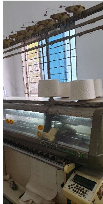
Figure 10.3 Flat knitting machine Source: Author (2020) in field visit of case study units
