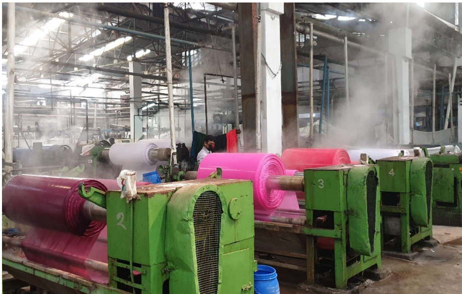
Figure 10.11 machines used for dyeing in Woven-dyeing textile unit Source: Author (2020) in field visit of case study units
