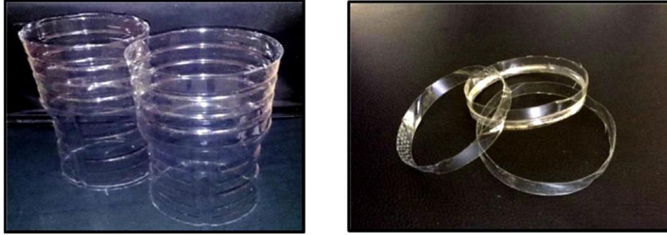
Figure 5. Ring-shaped plastic fibres used for improved concrete beam performance [31]
