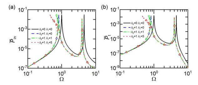
630 **Fig. 13.** Effects of the inerter-based nonlinear joint on (a) the time-averaged input power  $\bar{P}_{in}$ , and (b) the time-631 averaged transmitted power  $\bar{P}_t$  when the inerter-based joint is added at Q ( $\mu = 1, \gamma = 1, \kappa = 10, \zeta_1 = \zeta_2 =$ 632 0.01,  $F_0 = 0.05$ ).
