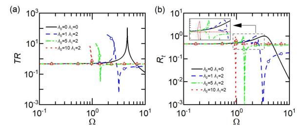
562 **Fig. 10.** Effects of the inerter-based nonlinear joint on (a) the force transmissibility  $T_R$ , and (b) the time-averaged 563 power transmission ratio  $R_t$  when the inerter-based joint is added at P ( $\mu = 1, \gamma = 1, \varkappa = 10, \zeta_1 = \zeta_2 =$ 564 0.01,  $F_0 = 0.05$ ).
