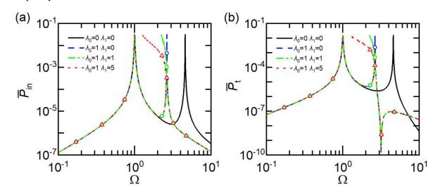
448 **Fig. 6.** Effects of the inerter-based nonlinear joint on (a) the time-averaged input power  $\bar{P}_{in}$ , and (b) the time-449 averaged transmitted power  $\bar{P}_t$  when the inerter-based joint is added at P ( $\mu = 1, \gamma = 1, \kappa = 10, \zeta_1 = \zeta_2 = 0.01, F_0 = 0.05$ ).
