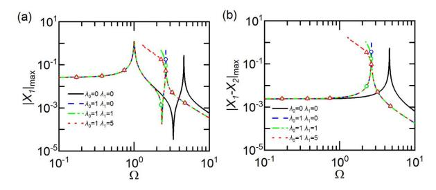
422 Fig. 5. Effects of the inerter-based nonlinear joint on (a) the response amplitude of mass  $m_1$ , and (b) the relative 423 response of masses  $m_1$  and  $m_2$  when the inerter-based joint is added at P ( $\mu = 1, \gamma = 1, \kappa = 10, \zeta_1 = \zeta_2 =$ 424 0.01,  $F_0 = 0.05$ ).
