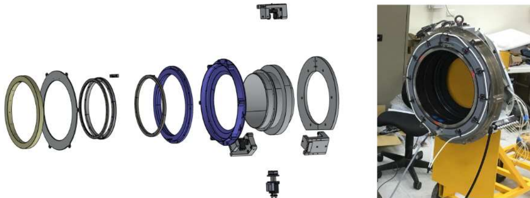
Figure 1. Left: Exploded view of the half-wave plate rotator (minor components excluded). Right: Assembled half-wave plate rotator in the receiver room of the Large Millimeter Telescope in Mexico.
