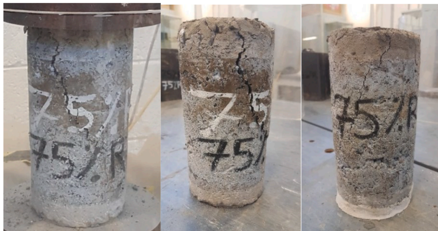
Fig. 10. Failure mode for RuRCC75% cylinders (mode of failure is not very clear).
