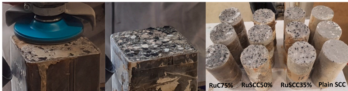
Fig. 5. Surface preparation/grading for the confined and unconfined specimens.
