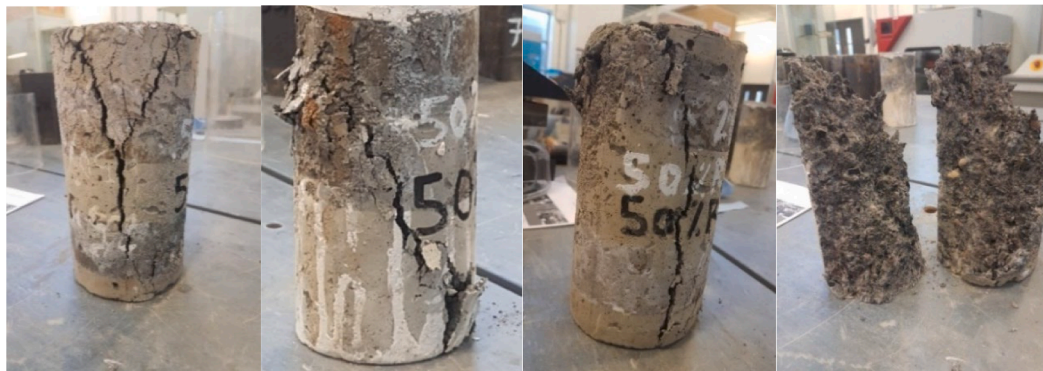
Fig. 9. Failure mode for RuSCC50% cylinders (Shear, Cone and Shear, or Cone and Split failure).
