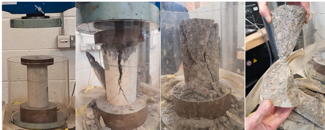
Fig. 7. Failure mode for unconfined Plain SCC cylinders (Cone failure).
