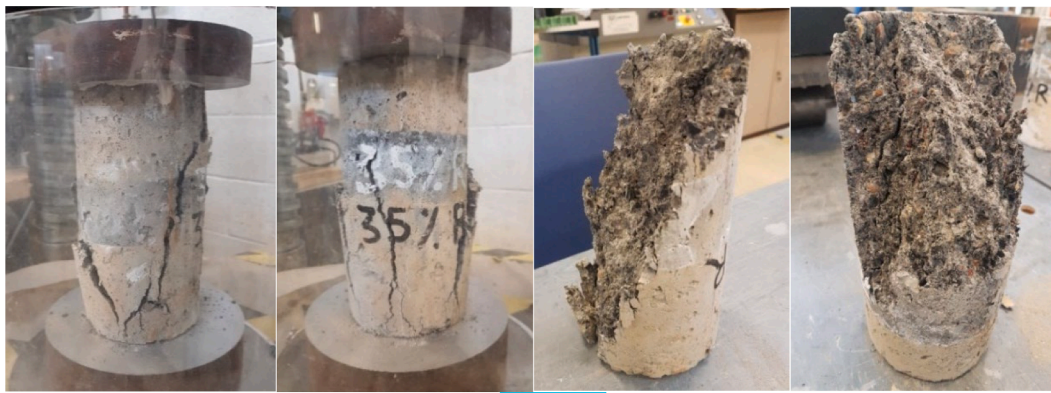
Fig. 8. Failure mode for RuSCC35% cylinders (Shear, or Cone and Shear failure).
