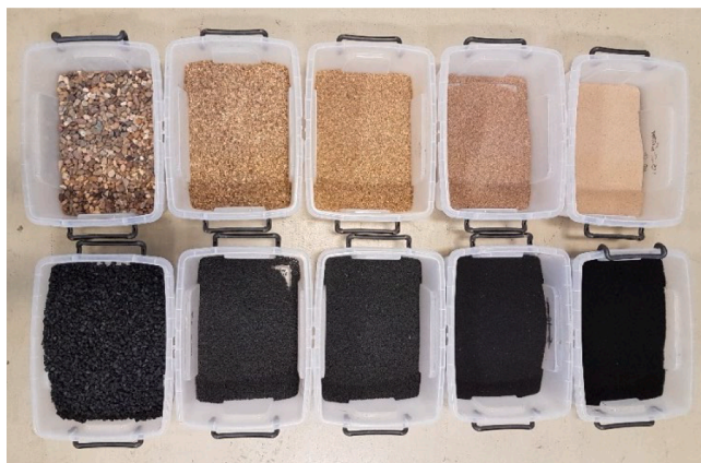
Fig. 2. Graded rubber and mineral aggregates prepared for a RuSCC mix.
