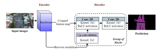
Fig. 3. Unet architecture illustration. Backbone network is chosen from state-of-art model, plays a role as encoder to exploit feature in multi-scale. Decoder consist of up-convolution and 2D convolution recover original resolution of feature map
