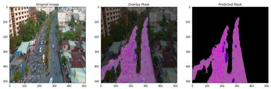
Fig. 10. Prediction mask produced by Unet + Inception backbone on Saigon Aerial dataset
