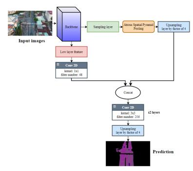
**Fig. 4.** DeeplabV3plus architecture. Atrous Spatial Pyramid Pooling is a sequence of parallel Atrous convolutions with different rates. By adusting filter's rate, multi-scale information is expoilted significantly
