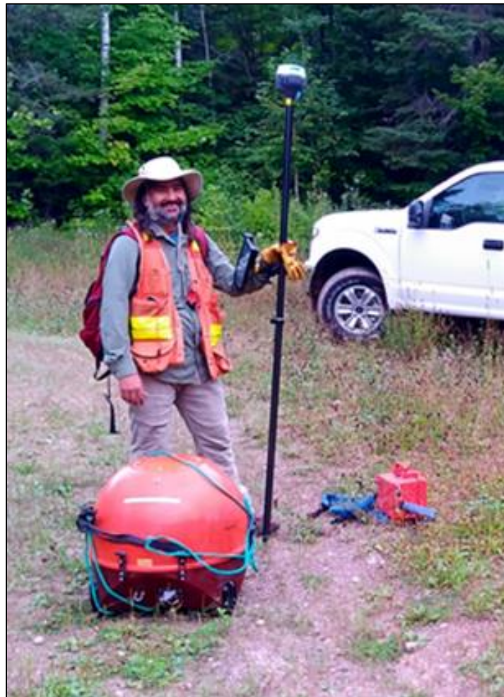
Figure 16 – ELF-EM system on site in New Brunswick. The receiver coil is in front of the operator while the survey console is to their right. A 15-meter data cable would be attached between the two before surveying began. The system in the operators' hand is a DGPS solution not required for the ELF.
