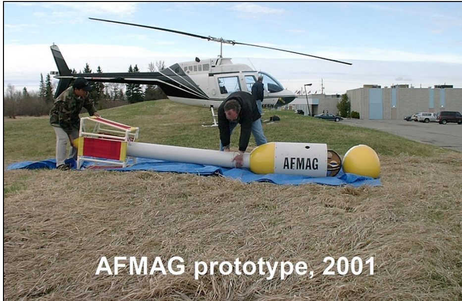
Figure 15 – Photo of an AFMAG prototype which would lay the groundwork for ZTEM surveying (airborne ELF). Photo was modified from Legault (2012).
