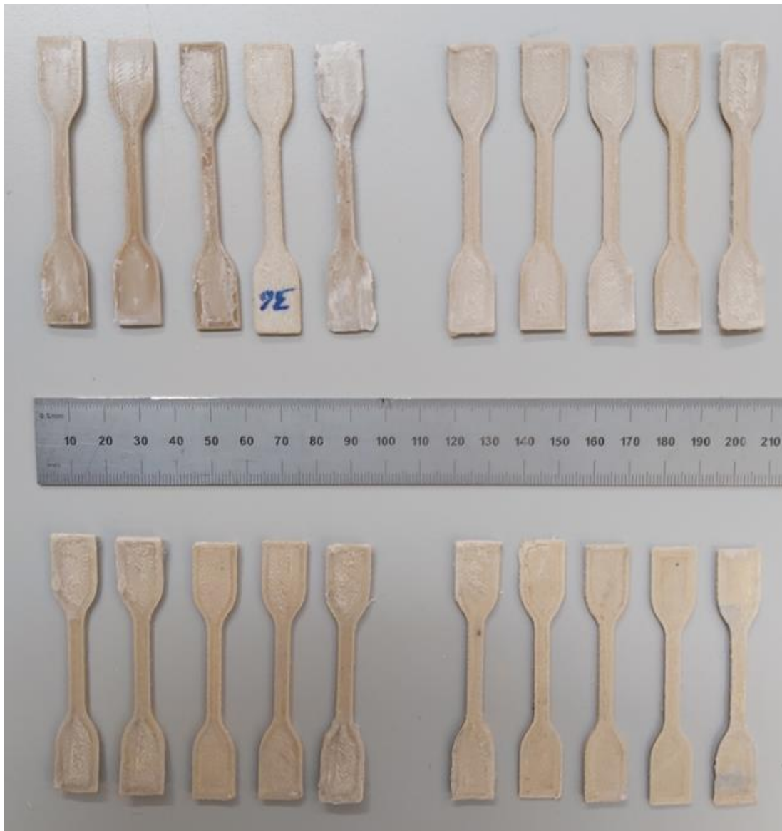
Figure 10 Tensile testing samples of PEEK nanocomposites prepared at optimized conditions via SpiderBot FFF 3D printer
