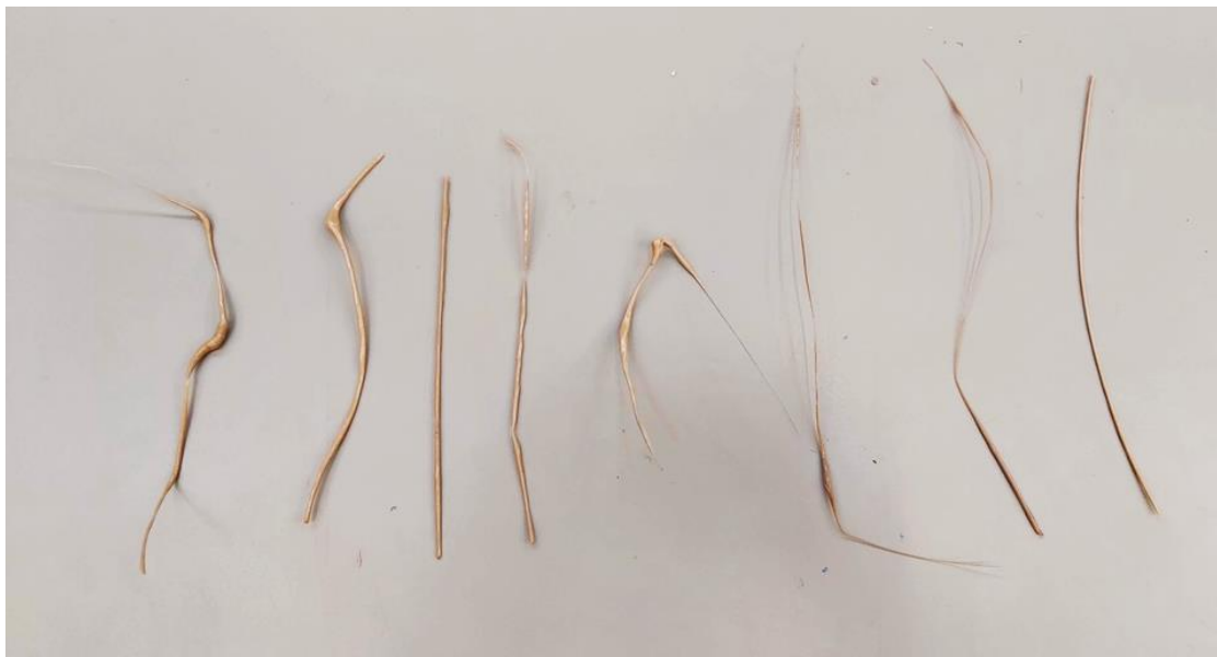
Figure 20 Non-uniform diameter of PEEK nanocomposite filaments obtained during optimisation via 3devo desktop extruder
