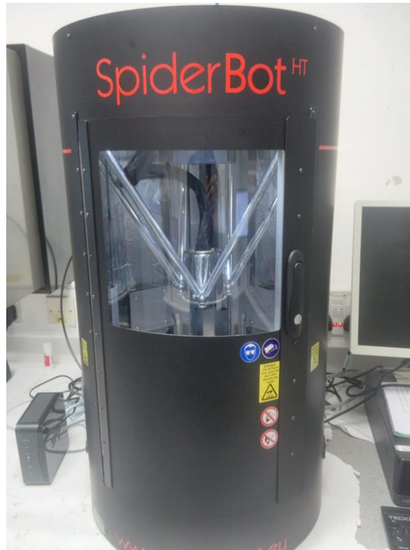
Figure 8 SpiderBot HT commercial FFF 3D printer for printing PEEK and its composite samples
