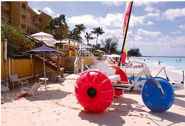
Fig. 13b. Marriott Beach Resort shoreline November 2012. Note the wooden steps onto the beach which indicate long-term reduction in beach volume.
