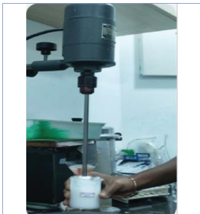
[Table/Fig-1]: Sol preparation by constant stirring.
