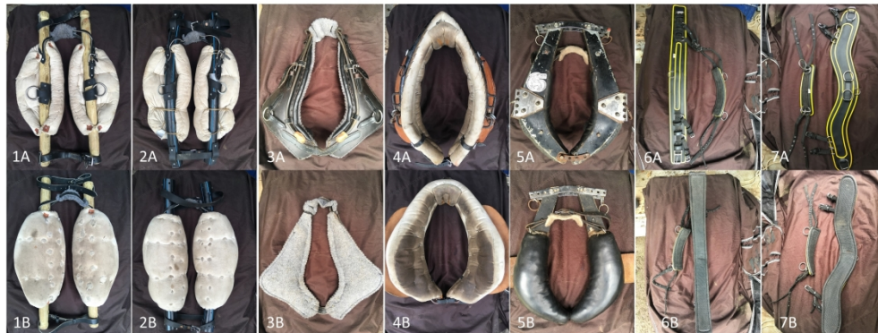
Figure 1. Seven collars tested: collar 1: manufactured using canvas for external padding, wool for internal padding and fence post as hames. Collar 2: similar with collar 1 but using 50 mm black water pipe for the hames. Collar 3: manufactured externally with natural leather and internally with felt, having natural wool as padding material and metal hames. A leather bridge keeps the two parts together of the collar at the bottom. Collar 4: made of canvas and rawhide, filled with natural wool and straw, with curved metallic hames with adjustable hitching point. Collar 5: manufactured with large plywood hames, padding area of natural leather filled with natural wool. Collars 6 and 7: manufactured with beta/biothane/synthetic leather, and filled with sponge. A = front view and B = rear view.
