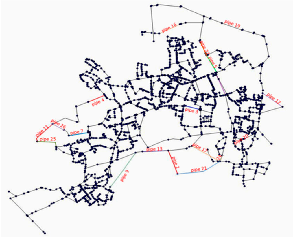
Figure 1. EPANET model for the WDN of a Dutch city, with indication of the pipes considered to be out of service in the 18 critical scenarios.
