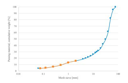
Table 3. Results of the conformity test: detail data for the grading curve of recycled aggregates from CDW.
