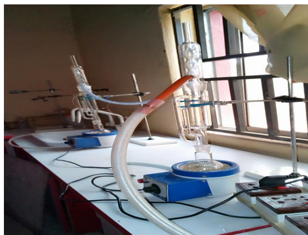
Figure 2 – Experimental apparatus for oil extraction
