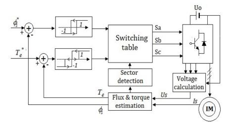
Figure 1. Basic DTC block diagram.
