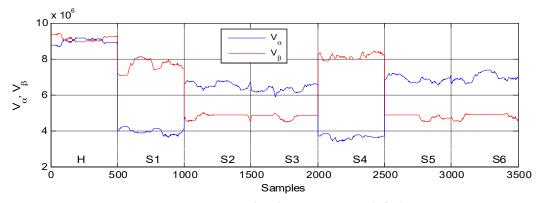
Figure 5. Feature extraction under short-circuit switch fault occurrence.
