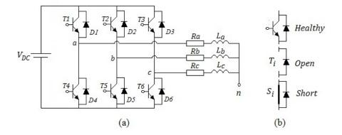
Figure 2. Diagram of a VSI feeding three-phase induction motor (a) and typical faults (b).
