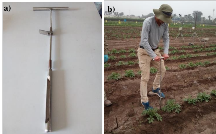
Figure 3.2: Punching soil sampler (a); obtaining the soil sample in the field (b).
