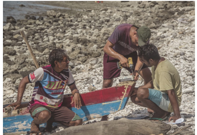
Plate 7. Solar-powered GPS unit (PDS-tracker) being installed on a fishing boat.
