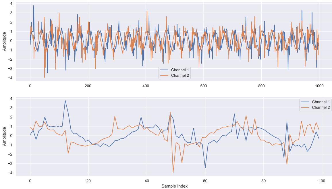
Figure 4.1. 1000 Samples and 100 Samples of Simulated Data With Random Interference: n = 2 , \sigma_{eps} = .1 , \sigma_r = 1 , p = .33
