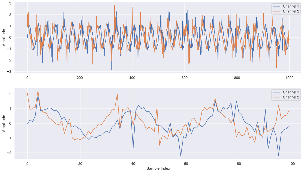
Figure 4.5. 1000 Samples and 100 Samples of Simulated Data With Random Directed Interference: n = 2 , \sigma_{eps} = .1 , \sigma_r = 1 , p = .33 , \theta_r = \frac{\pi}{2}
