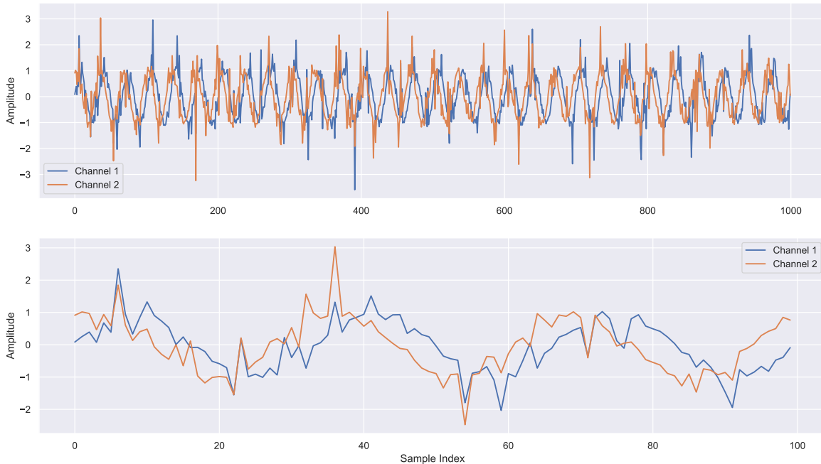
Figure 4.6. 1000 Samples and 100 Samples of Simulated Data With Random Directed Interference: n = 2 , \sigma_{eps} = .1 , \sigma_r = 1 , p = .33 , \theta_r = \frac{3\pi}{4}
