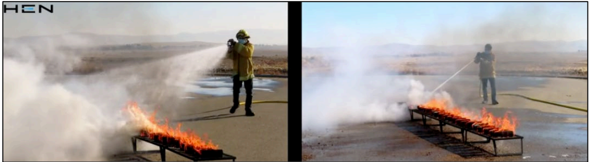
Figure 11. Demonstration of the HEN Smoothbore Nozzle vs. Conventional 3/8 Smoothbore Nozzle. Source: HEN at https://hennozzles.com (2022).
