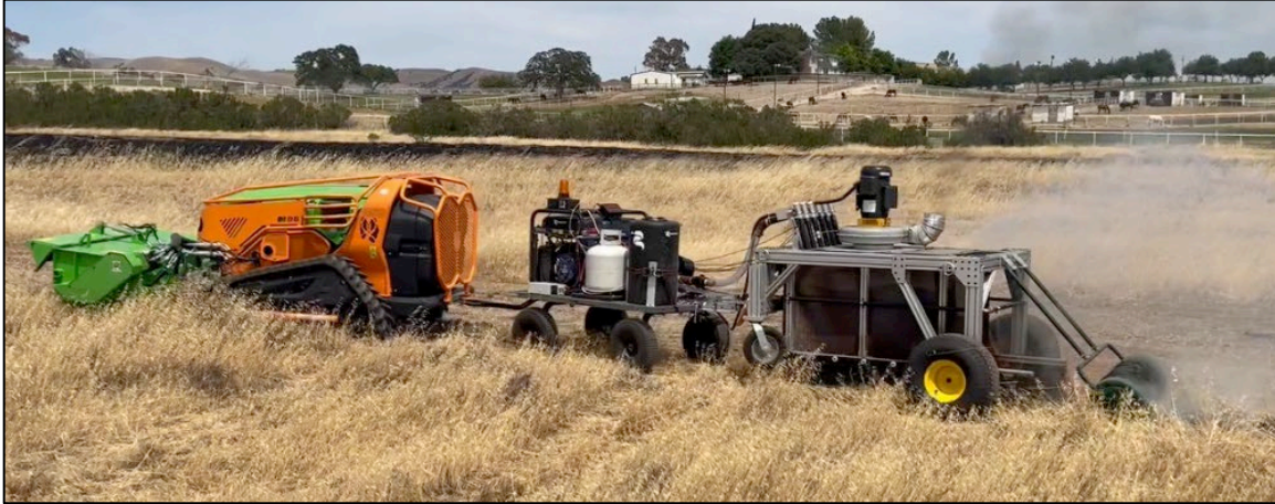
Figure 13. Demonstration of Burnbot Being Utilized to Create a Fire Break in a dense Dry Environment aboard Camp Roberts, CA (2022).
