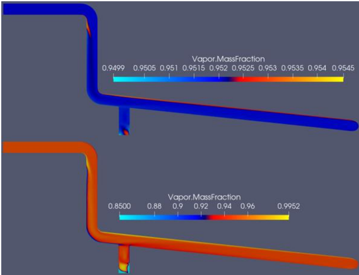
Figure 65. Vapor mass fraction contour for X = 95.19\% , d_{\text{droplet}} = 1 \mu\text{m} (top) and 10 \mu\text{m} (bottom) at inlet
