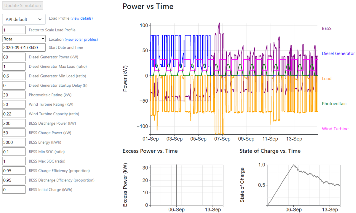
Figure 21. Microgrid Planning Tools Power Flow Simulation Web Interface. Source: Reich (n.d.)
