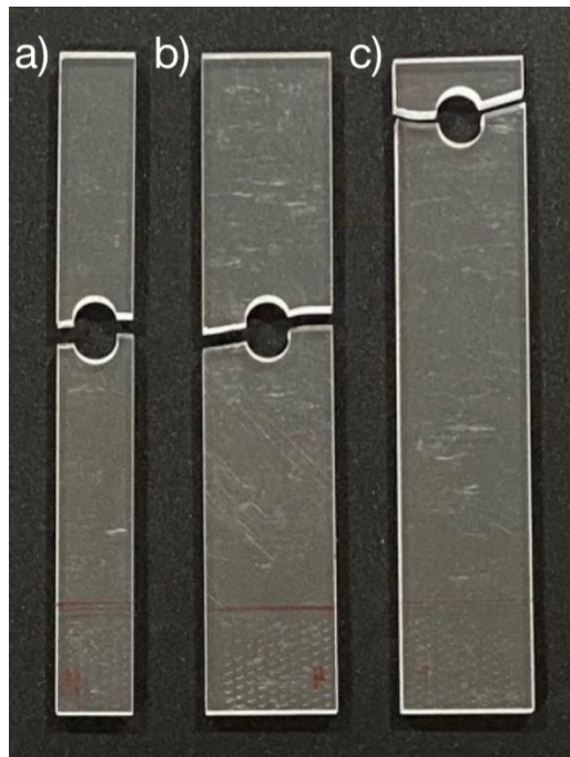
Figure 31. Specimen fracture with 6 mm bolt: a) P1, b) P2, and c) P3
