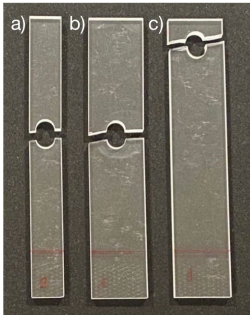
Figure 30. Specimen fracture with 8 mm bolt: a) P1, b) P2, and c) P3
