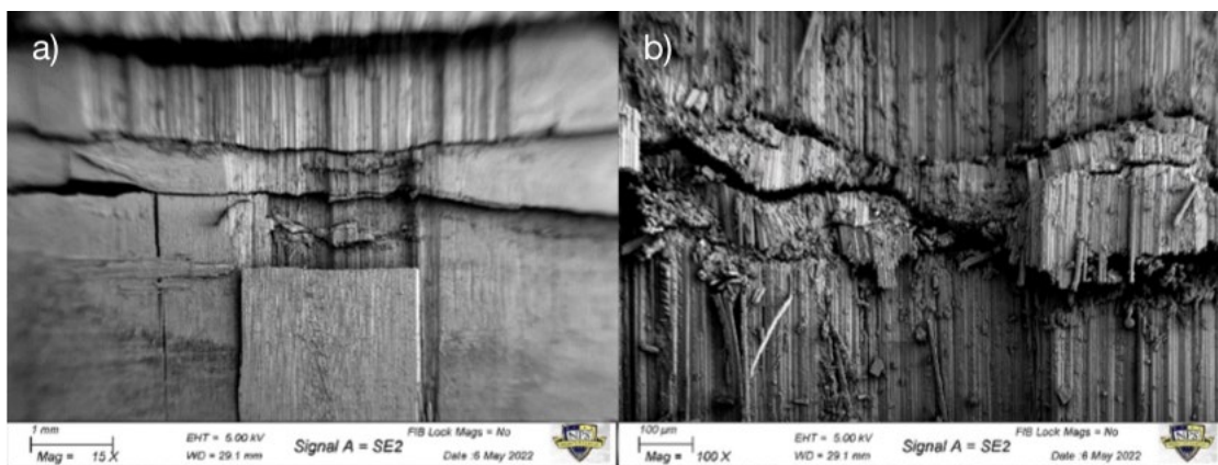
Figure 65. SEM front view of section A (above contact surface) from C1 sample: a) lower magnification and b) higher magnification
