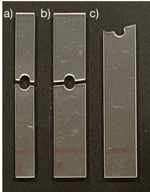
Figure 32. Specimen fracture with 5 mm bolt: a) P1, b) P2, and c) P3
