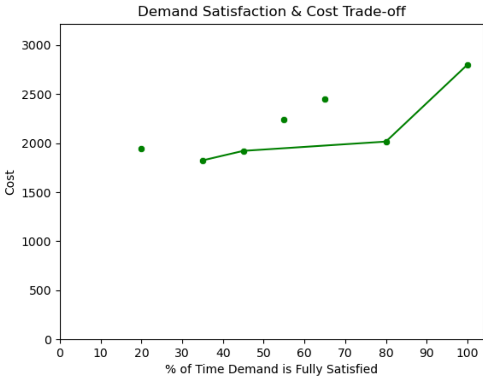
Figure 4.4. Plot showing the trade-off between demand satisfaction and cost. In this case, the maximum amount of supplies that can be prepositioned the terminal nodes is the expected demand across scenarios.
