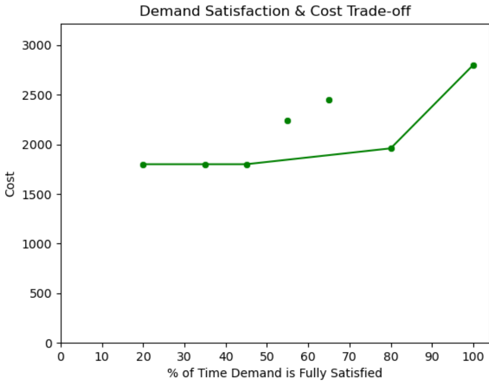
Figure 4.6. Plot showing the trade-off between demand satisfaction, cost, and gap. No prepositioning limit at terminal nodes.
