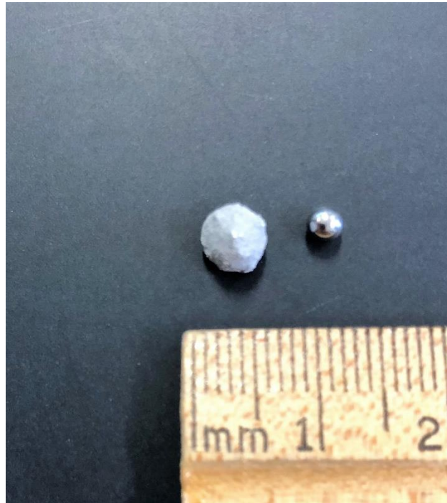
Figure 13. Aluminum sintered stainless steel milling ball (left) and original milling ball (right)
