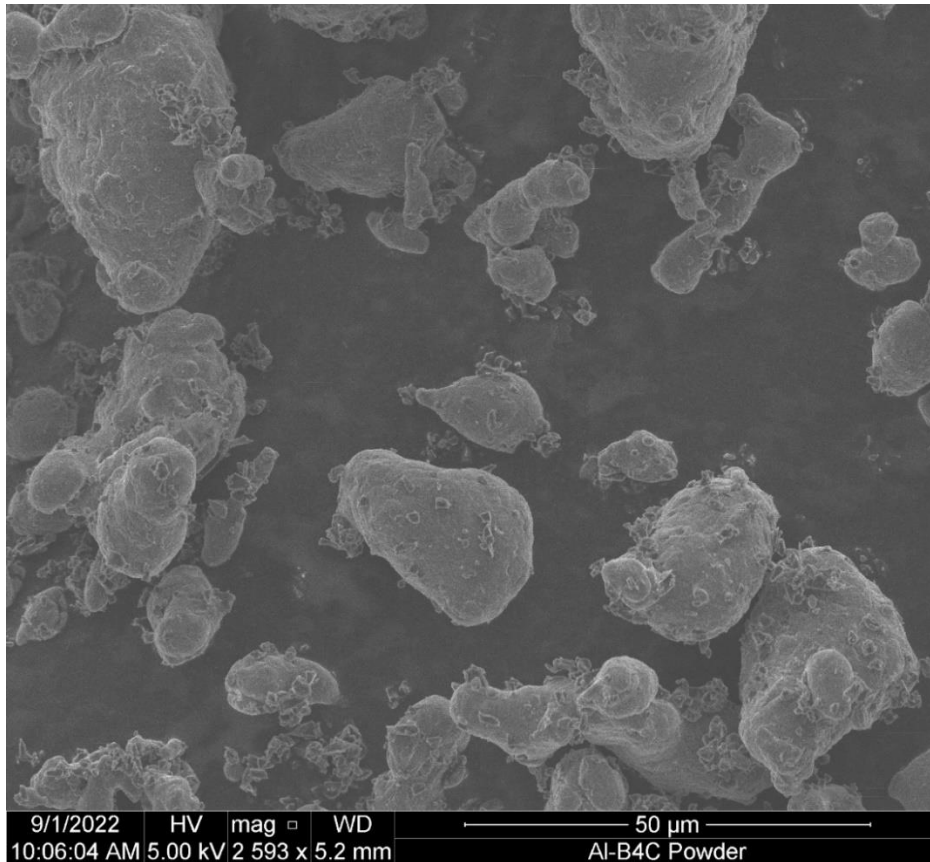
Figure 19. Aluminum and B 4 C powder post HEBM
