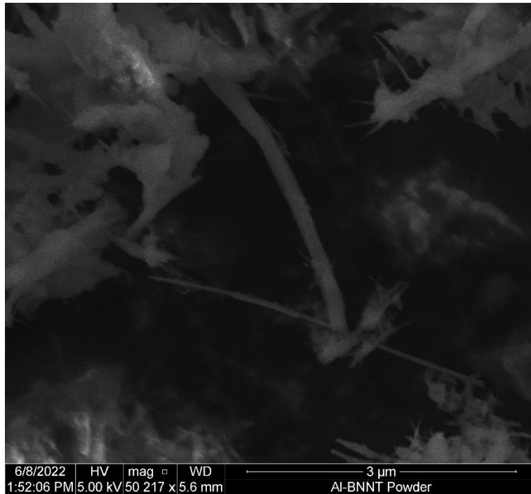
Figure 11. Various morphologies and agglomerations of BNNTs under the SEM
