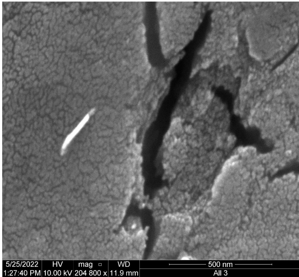
Figure 40. SEM image showing a chopped BNNT
