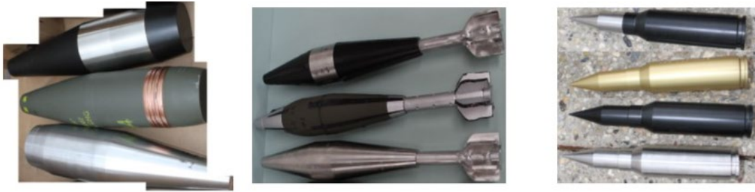
Fabricated surrogate, purchased replica, and fabricated replica of (left) 155 mm HE M107, (middle) 81 mm mortar, and (right) 25mm and 20 mm cartridges.
