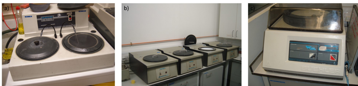
FIGURE 3.22. Pictures of the grinders/polishers at the School of Physics (IAC), University of Bristol. From the left (a) grinder/polisher Buehler Metaserv with two rotors with exchangeable coarsest papers. ECOMETs polishers using a diamond paste are shown on picture (b). From left to right the grade of Diamond paste are 3 \mu m, 1 \mu m, 0.25 \mu m and 0.1 \mu m. Vibro-Polisher used for the final polishing step of the sample, with colloidal silica ( 20 nm diam.) is shown on picture (c).
