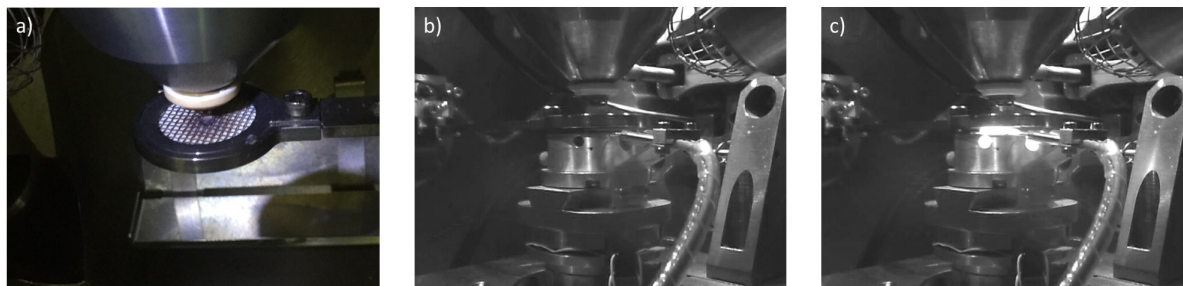
Figure 6.2: Images of the FEI Quanta 200 FEG ESEM chamber taken at different temperatures: (a) room temperature, (b) 300°C, and (c) 800°C.
