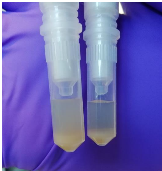
Figure 3.1. Visual quality assessment of viable extract. Left hand side: poorly processed extract appears as turbid. Right hand side: the extract has distinct layers and a clear supernatant; therefore, it has been correctly bead-beaten.
