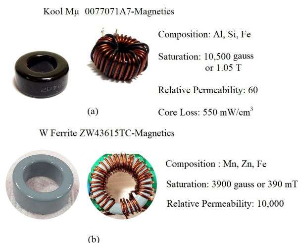
Figure 6. Comparison of magnetic properties: (a) Kool \mu powdered-iron toroid (0077071A7); (b) W-Ferrite toroid (ZW43615TC).
