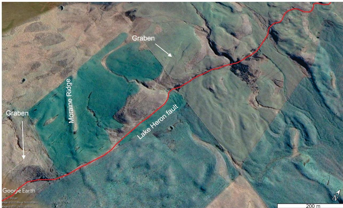
Figure 2-11. Moraine deposits are displaced by the Lake Heron fault. No lateral offset of the displaced moraine ridge is found at the southwest part of the image. Two crestal grabens are formed in the moraine deposits to the north of the South Branch Ashburton River. Grabens are in the hanging wall of the fault.
