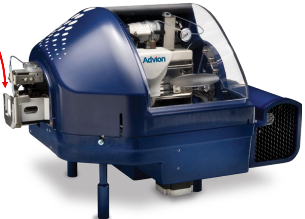
Figure 9: An Advion ESI source set-up is displayed. The ESI chip is slotted into an ESI-carrier located at the front of an autosampler, samples are aspirated and sequentially sprayed through the nozzles on the chip.
